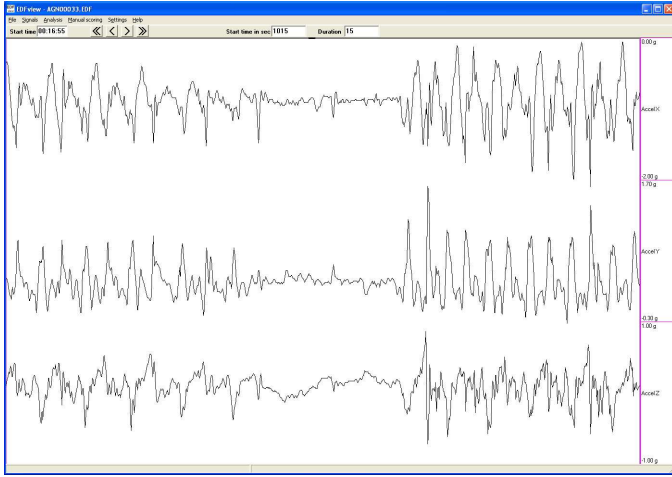
Fig. 1. A typical tri-axial accelerometer multi-plot showing 15 seconds of data, 75 samples per second (data set courtesy of Prof. Jun Jo, Griffith University, Australia)
